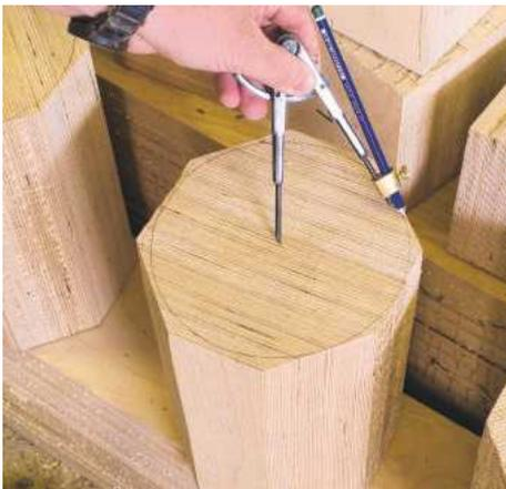
▲ Pic.4 He likes to get as close to his finish size as possible, because it's easier to cut away the wood with the saw than to turn it. He picks the middle strip of the ply and draws a circle to find the centre
